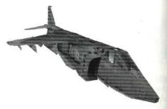
of more than 90 degrees. Known as "thrust vectoring", this technique is used for vertical takeoff and landing, and hovering. It can also be used in combat to increase the aircraft agility – this is known as "viffing" (Vectoring In Forward Flight), and you'll learn how to do this later in this section of the manual.
